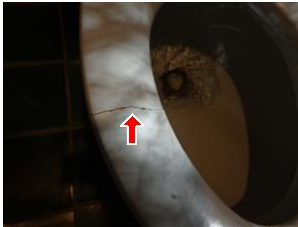
6.0 Picture 5 cracked seat
