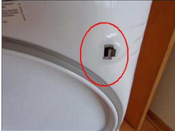
6.0 Picture 4 catch loose in door
